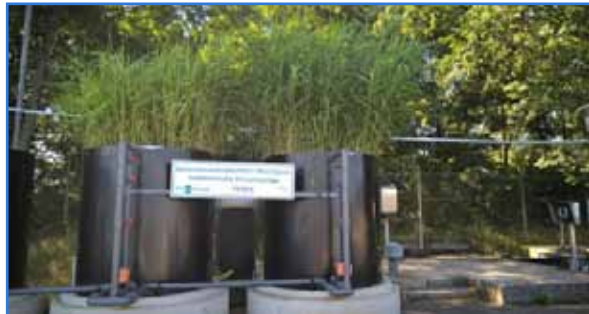
Figure 2: RSF test facility to investigate the effectiveness of RSF as an additional purification stage for WWTPs (Source: IHPH)
